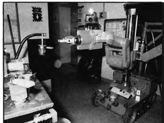
Robot Hard Herman training to take a core sample.
